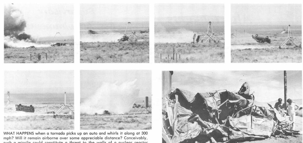
such a missile could constitute a threat to the walls of a nuclear reactor structure. In tests being run for the Electrical Power Research Institute in Area III, it was learned that the 300 mph flying auto would probably sail several hundred feet before touching down. Rocket sled provided desired velocity, and auto became airborne after sled was suddenly braked. At right, Bob Lucas (2323) and test engineer Kathleen McCaughey (1535) examine remains.
